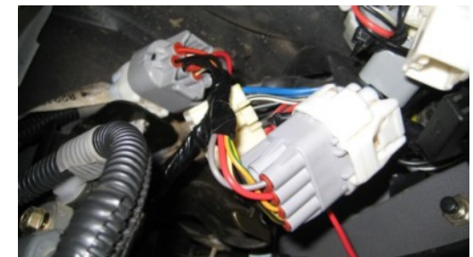
Connect the cruise T-patch pedal harness between the throttle pedal & the vehicles harness.
