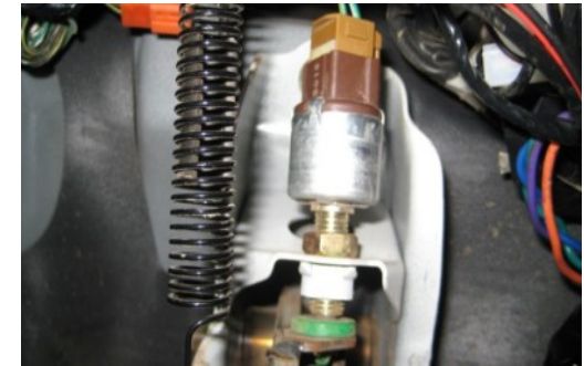
Connect brake T-patch to factory brake switch.
