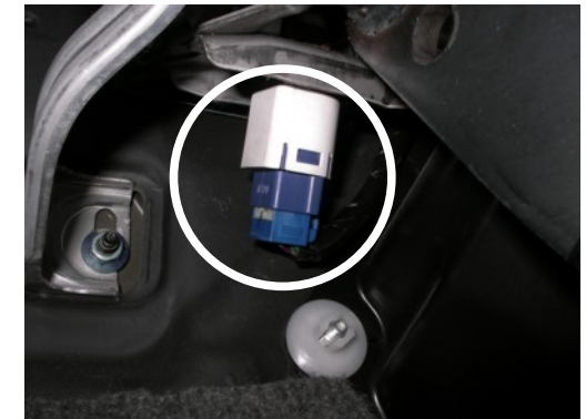
Connect brake T-patch to factory brake switch.
