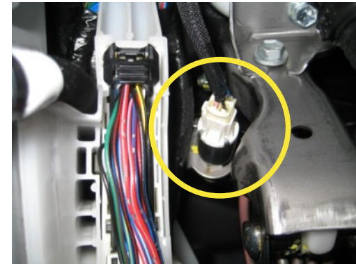
Connect clutch T-patch to factory clutch switch. NOTE; The Yellow wire should match with the Pink/Black wire.
