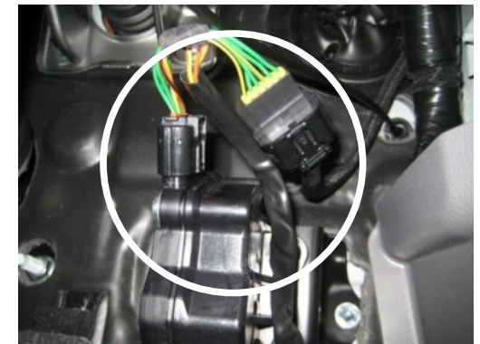
Connect the cruise T-patch pedal harness between the throttle pedal & the vehicles harness.
